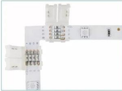
3. The contacts of the light bar are inserted into the connector to ensure that the contact points are fitted.
