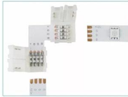
2. Open the L shape connector, the strip light is aligned with the + pole of the connector.
