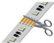
1-1: Cut LED Strip along the cuttable mark
