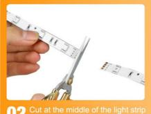
02 Cut at the middle of the light strip where there are solder joints.
